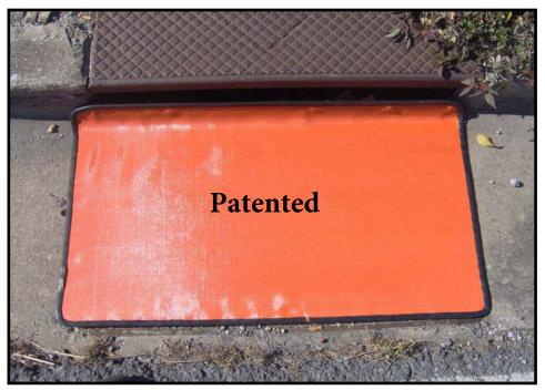
The Suntree Technologies Gr8-Protector TM is manufactured to filter stormwater runoff during construction until final stabilization is achieved. The Gr8-Protector is secured to the grate with the applicable fastening system (usually JH-67M "patented") that is supplied with each inlet protector. The fabric shall meet the specifications below and be reinforced with an expanded steel backing.
